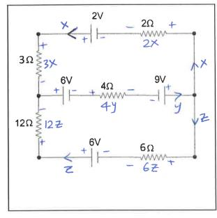
5. Write down the loop rule equation, for the bottom loop, and simplify.
